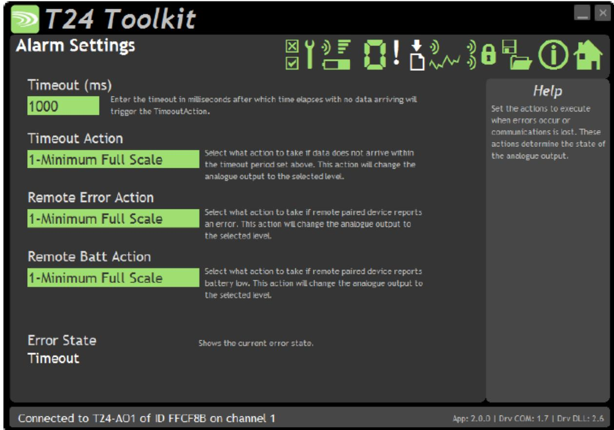
Here you can set the action to take when certain errors occur. The actions are applied when the errors occur and if more than one error is present the actions are applied with the following priorities:
