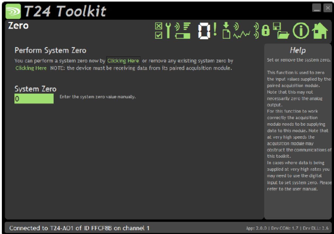
System zero allows you to zero the input. The system zero value is subtracted from the input value before it is used to determine the analog output to apply.
